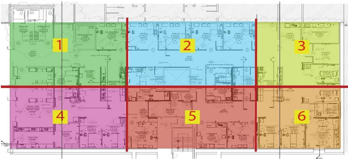
Figure 5-4 – Zones for overhead MEP rough-in phase
